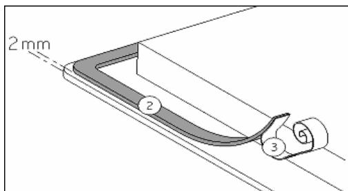
Stick the gasket (2) two millimeters from the external edge of the glass, after removing the protection sheet (3).
